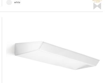
Wall lighting fixture for interiors, with direct and indirect light emission. Pickled sheet metal wall bracket in polyacrylic paint. Extruded aluminium structure in white, black, bronze, mat brass or titanium polyacrylic paint. Extruded acrylic diffusers with opaline finish.
