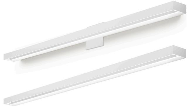
Ceiling or wall lighting fixture for interiors, with direct and indirect light emission. Pickled sheet metal structure in white, bronze or mat brass polyacrylic paint, or with gold leaf coating, or in polished stainless steel. Specular aluminium reflector. Cover in brass with white, bronze or mat brass polyacrylic paint, or with gold leaf coating, or with galvanic chrome plating. Extruded polycarbonate diffuser with opaline finish.
