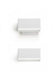
Wall lighting fixture for interiors, with direct and indirect light emission. Body in extruded aluminium and cover in pickled sheet steel, with white, black, bronze, mat brass or titanium polyacrylic paint. Wall mounting bracket in bent steel sheet. Opal polycarbonate diffuser screens.
