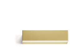
Wall lighting fixture for interiors, with direct and indirect light emission. Body in extruded aluminium and cover in pickled sheet steel, with white, black, bronze, mat brass or titanium polyacrylic paint. Wall mounting bracket in bent steel sheet. Opal polycarbonate diffuser screens.
