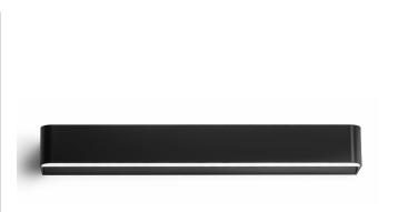
Wall lighting fixture for interiors, with direct and indirect light emission. Body in extruded aluminium and cover in pickled sheet steel, with white, black, bronze, mat brass or titanium polyacrylic paint. Wall mounting bracket in bent steel sheet. Opal polycarbonate diffuser screens.
