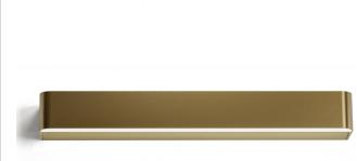
Wall lighting fixture for interiors, with direct and indirect light emission. Body in extruded aluminium and cover in pickled sheet steel, with white, black, bronze, mat brass or titanium polyacrylic paint. Wall mounting bracket in bent steel sheet. Opal polycarbonate diffuser screens.
