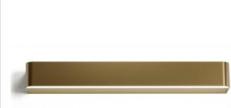
Wall lighting fixture for interiors, with direct and indirect light emission. Body in extruded aluminium and cover in pickled sheet steel, with white, black, bronze, mat brass or titanium polyacrylic paint. Wall mounting bracket in bent steel sheet. Opal polycarbonate diffuser screens.
