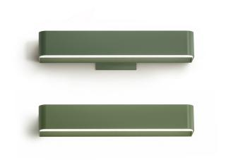
Wall lighting fixture for interiors, with direct and indirect light emission. Body in extruded aluminium and cover in pickled sheet steel, with white, black, bronze, mat brass or titanium polyacrylic paint. Wall mounting bracket in bent steel sheet. Opal polycarbonate diffuser screens.
