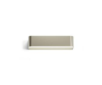
Wall lighting fixture for interiors, with direct and indirect light emission. Body in extruded aluminium and cover in pickled sheet steel, with white, black, bronze, mat brass or titanium polyacrylic paint. Wall mounting bracket in bent steel sheet. Opal polycarbonate diffuser screens.
