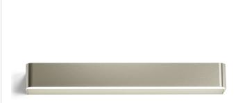
Wall lighting fixture for interiors, with direct and indirect light emission. Body in extruded aluminium and cover in pickled sheet steel, with white, black, bronze, mat brass or titanium polyacrylic paint. Wall mounting bracket in bent steel sheet. Opal polycarbonate diffuser screens.
