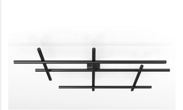
Ceiling lighting fixture for interiors, with direct and indirect light emission. Pickled sheet metal ceiling bracket in polyacrylic paint. Pickled sheet metal wall plate in polyacrylic paint. Extruded aluminium structure in white, mat black, bronze, mat brass or titanium polyacrylic paint. Joints in turned brass and die-cast aluminium in polyacrylic paint. Die-cast aluminium end caps in polyacrylic paint.
