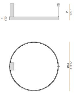
Ceiling or wall lighting fixture for interiors, with direct and indirect light emission. Pickled sheet metal ceiling or wall bracket in polyacrylic paint. Pickled sheet metal wall plate in polyacrylic paint. Bended extruded aluminium structure in white, black, bronze, mat brass or titanium polyacrylic paint.
